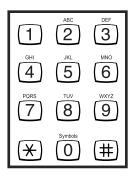
Each time you press **6**, the LCD display shows a different letter, first **M**, then **N** and **O**, and finally **6**.
